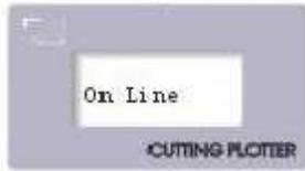
To switch the machine to offline mode press the online button (7).
