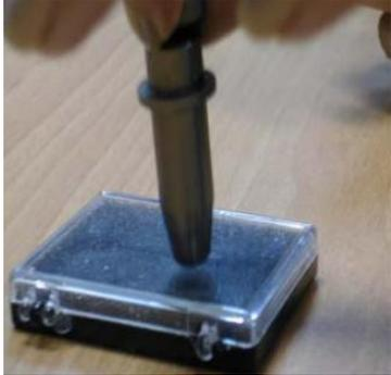
The blade is a consumable item and you’ll always get the best quality cut with a newer blade. Replace with a new blade when: 1) the tip is broken, 2) The cutting traces are not as good as they were, 3) The blade will not cut cleanly, even though the force/pressure has been increased.
