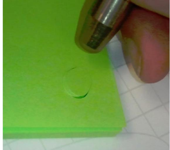
The goal for this test is to set the depth of the blade so that you can cleanly cut a circle out of a single sheet of paper, while barely leaving a scratch on the piece directly underneath it.
