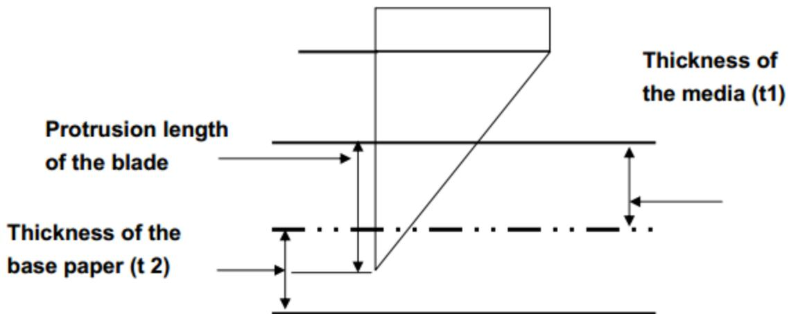
Length of protrusion =  $t_1 + t_2 / 2$ , but for your convenience you may just set it about 0.3mm ~ 0.5mm beyond the blade holder tip.
