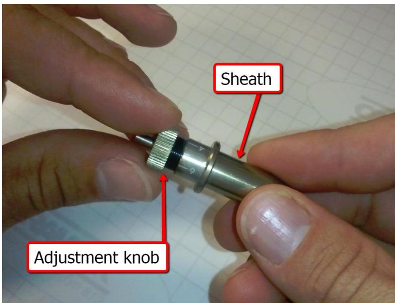
The Zencut blade holder uses a sheath and adjustment knob. When holding the blade-holder as shown in the image to the left; screwing the adjustment knob clockwise will expose more blade. Unscrewing it (counter-clockwise) will reduce the amount of blade exposed.
