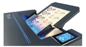
The Led light strip provides stable lighting conditions so that the camera can reliably read the QRcodes and registration marks regardless of the external lighting conditions. This leads to improved reliability during unattended operation of the cutter.
