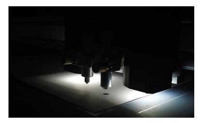
The FC-500VC uses a high resolution camera for accurate detection of registration marks (as small as 5 mm) and can see reg marks on both colored and transparent materials. The ability to scan small reg marks saves material, thus reducing production costs.
