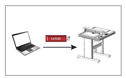
PLT-files saved on USB thumb drives (U-disk) can be used for direct output. This means that the FC-500VC can be used without being connected to a computer.
