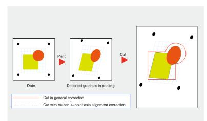
The Vulcan FC-500VC efficiently handles materials loaded on a slant and also compensates for size/shape distortions. Precise and accurate cuts are assured with our proprietary fourmark high-tech detection algorithm.
