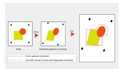
The Vulcan FC-700VC efficiently handles materials loaded on a slant and also compensates for size/shape distortions. Precise and accurate cuts are assured with our proprietary fourmark high-tech detection algorithm.
