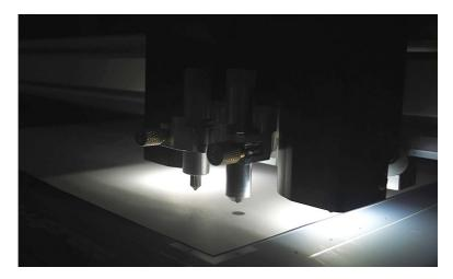
The FC-700VC uses a high resolution camera for accurate detection of registration marks (as small as 5 mm) and can see reg marks on both colored and transparent materials. The ability to scan small reg marks saves material, thus reducing production costs.
