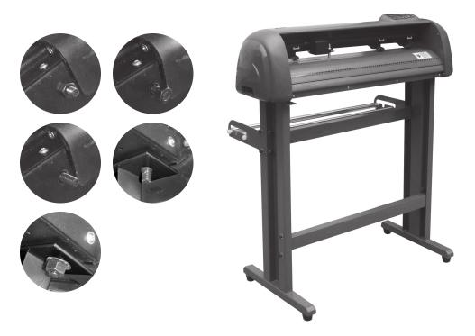
Take off the screw from bottom of machine, insert bolt to top of floor stand, then tighten the screw.
