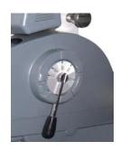
The roller nip adjustment quick-select notch system used on the RSC-820CLS roll laminator significantly simplifies adjusting the gap between rollers, making webbing and mounting easier.
