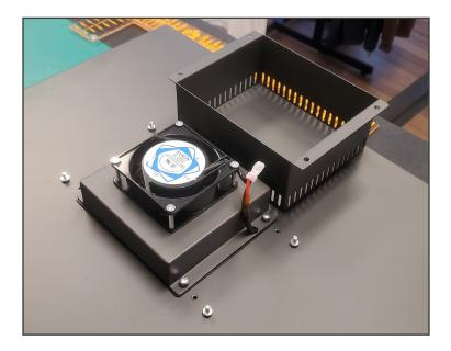
Fan filters might need to be changed every 3 to 6 months depending on how often you use your oven. Changing the filters will require you to remove 8 screws (4 from top cover, 4 from bottom assembly). The two filters can be removed from the underside of the bottom assembly.
