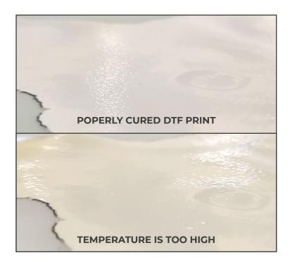
A properly cured DTF print will show a shiny, dry, orange peel texture. If your curing process shows fuzzy areas, they are not yet sufficiently cured. If the white orange peel texture starts to turn brown or the film starts to severely buckle, your temperature is too high. Low and slow curing tends to provide the best results. Placing a partially cured print back in the oven for additional curing is not a problem.
