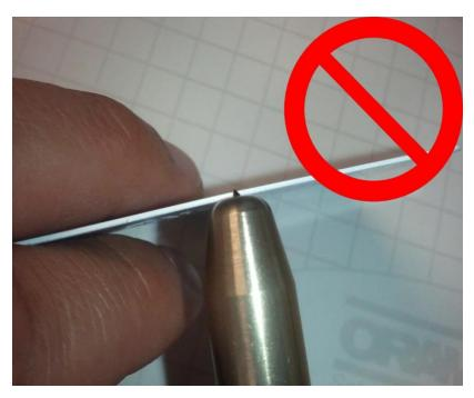
way through the thickness of the credit card. If the tip of the blade goes past or reaches the other side of the card as pictured to the left, then you have too much blade showing.
