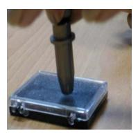
The blade is a consumable item and you'll always get the best quality cut with a newer blade. Replace with a new blade when: 1) the tip is broken,
